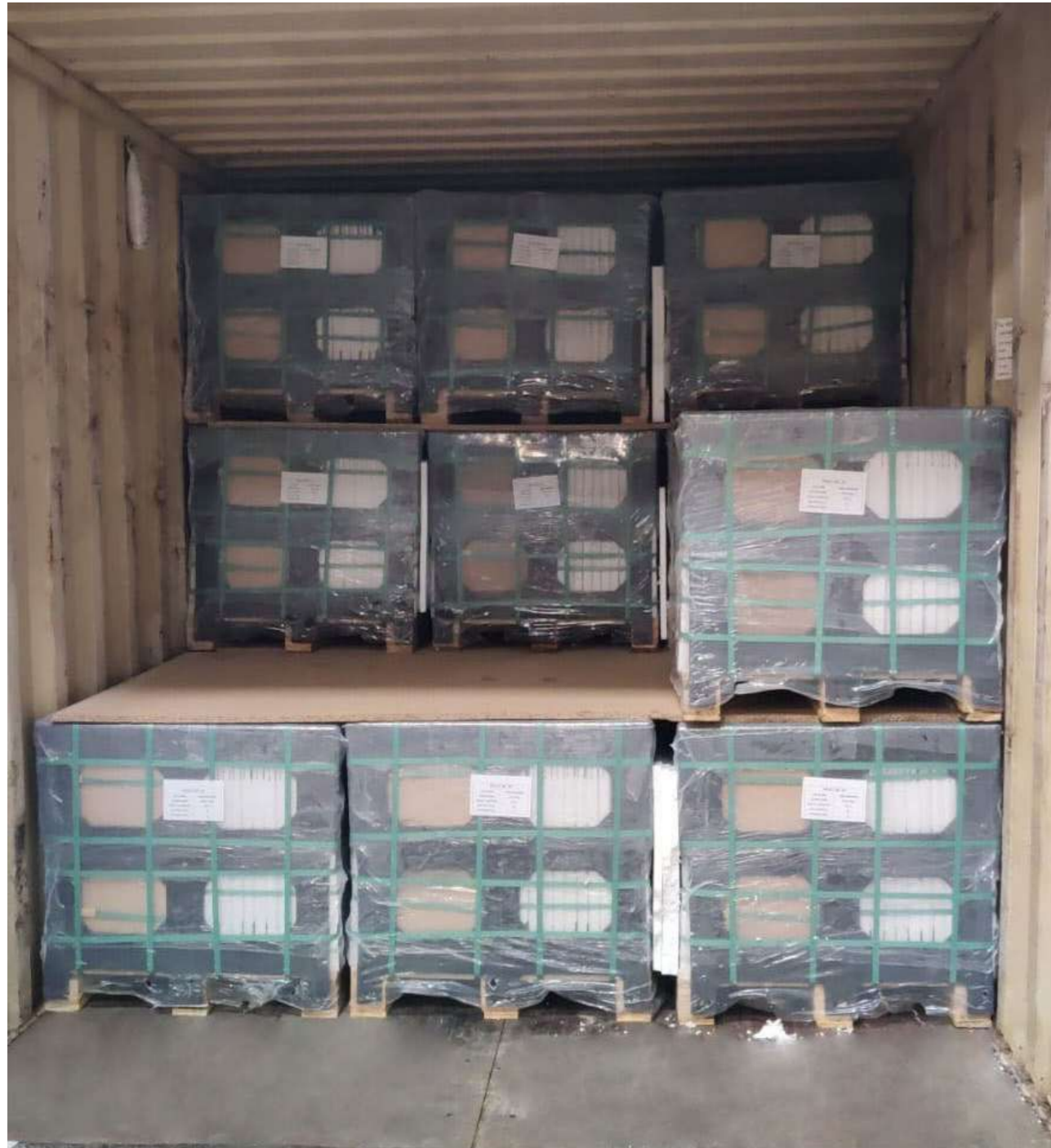
PLYWOOD BETWEEN EACH LAYER OF PALLET + POLYSTYRENE BETWEEN THE PALLET + HARD PLASTIC COVER ON EACH SIDES OF THE PALLET
